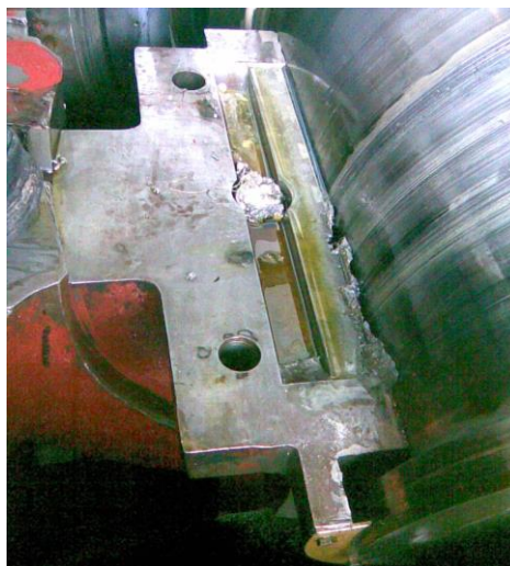
Fig. 17. Appearance of damage to the white metal on the sleeve
