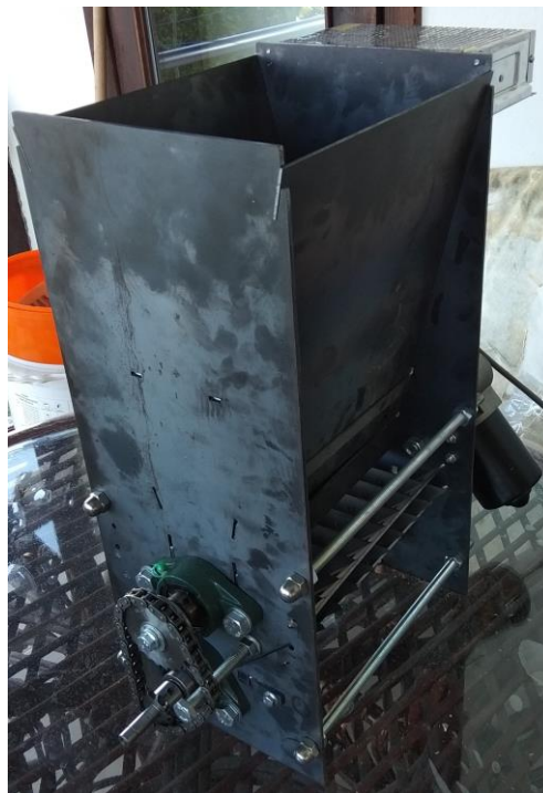
Fig. 1. Author concept and design of hazelnut unshelling apparatus
