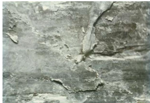
Fig. 4. Heavy adhesive wear (sealing)
