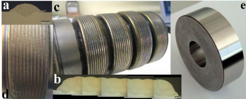
Fig. 6. Laser cladding of Vanadis23 powder on ring (20mm wide and 60mm in diameter) form C45 (ČI530) steel substrate: a) single layer; b) 3mm thick layer (with 30% overlapping); c) and d) single and double layer and e) after machining and grinding
