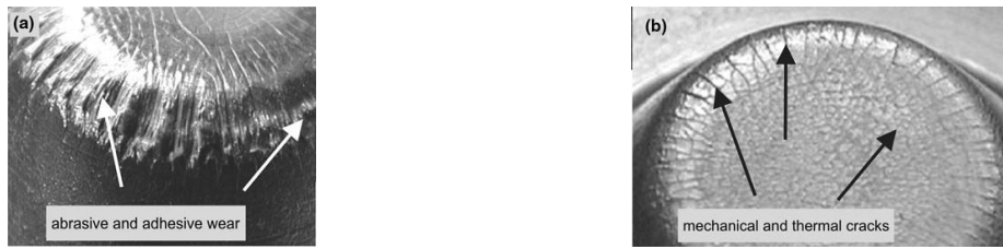
Fig. 3. Main wear mechanisms in examined forging tools in the mainly loaded regions [3]
