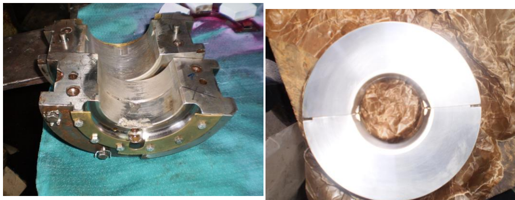
Fig. 19. Sliding bearing damage (left) and appearance of new "lemon" bearing (right)
