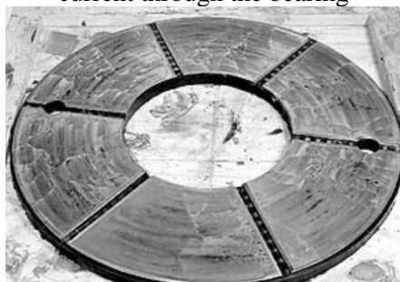
Fig. 7. Axial sliding bearing placental fatigue
