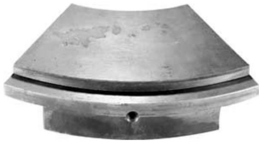
Fig. 9. Oxidation of the placenta due to contamination of lubricants with aggressive substances
